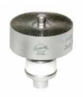
The 3CX6000A7/YU-148 high-mu, force air cooled power triode provides relatively high power output as an amplifier, oscillator or modulator at low plate voltages. The tube has a low inductance cylindrical filament stem structure which readily becomes part of a linear filament tank circuit for VHF operation. The grid provides shielding between the input and output circuits for grounded grid applications and conveniently terminates in a ring between the plate and filament terminals.
